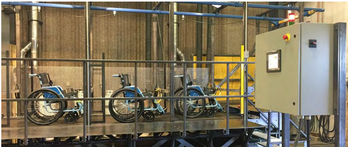
Figure 5: Whole-chair Durability Testing System at FWM
