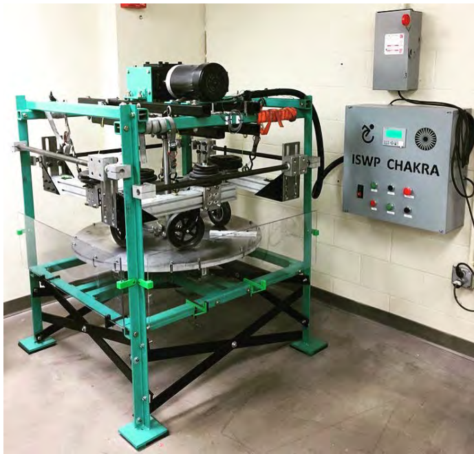
Figure 2: ISWP Castor Testing System also called as ISWP Chakra
