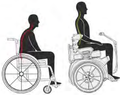
Figure 1. Posture and equilibrium control on active vs active powered wheelchair
