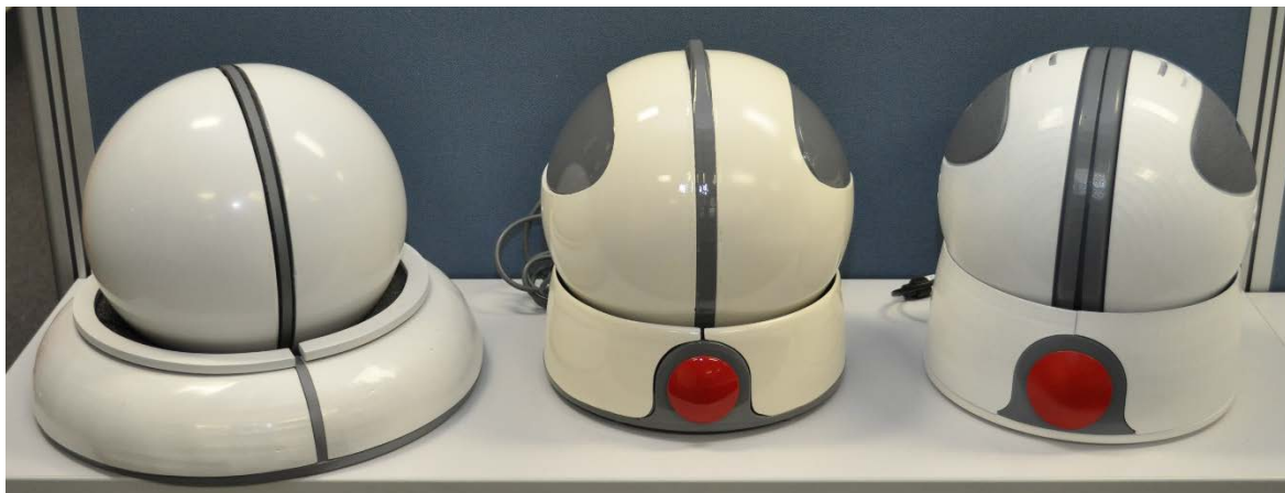
Figure 8: Different prototype gaming controllers that were manufactured during the project, from first concept (left) to final controller design (right)
