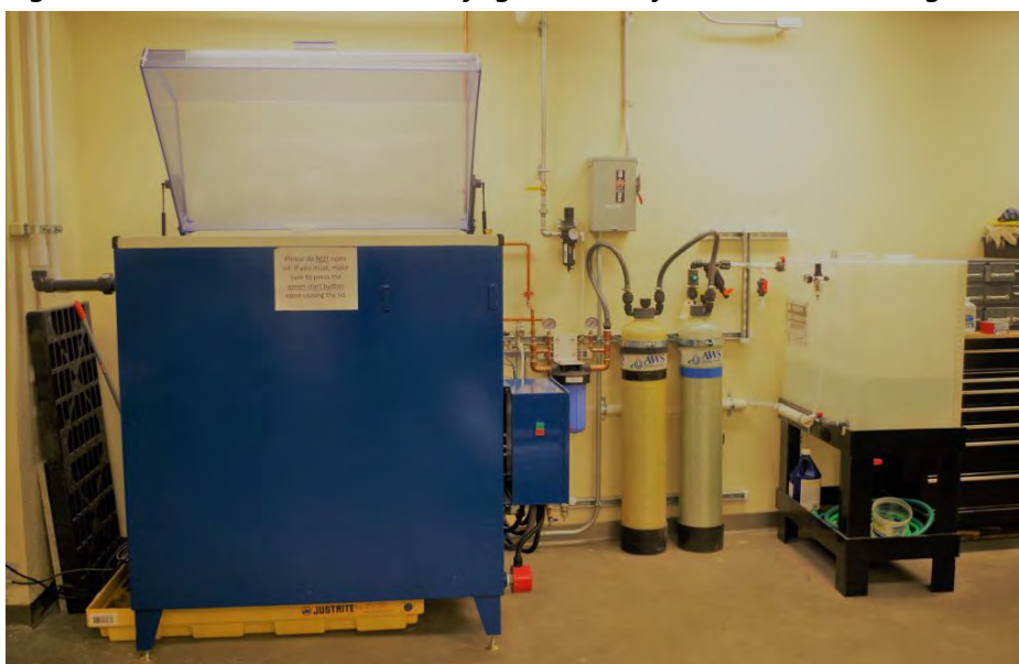
Figure 4: ASTM B117-based salt fog chamber for corrosion testing
